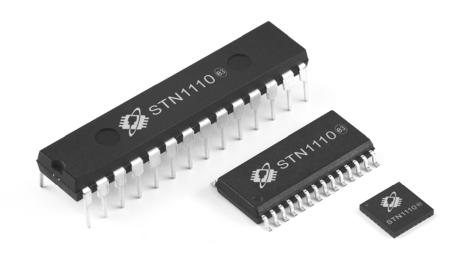
The IC supports all legislated OBD-II communication protocols, and features a sophisticated automatic protocol detection algorithm, ensuring compatibility with the widest range of vehicles. In addition to emulating the full ELM327 command set, STN1110 supports an extended command set that provides access to advanced functionality not available in the original ELM327, as well as faster data throughput on all protocols – sometimes by as much as 100%.
